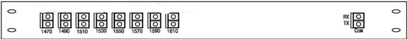
1u 19 Rack Mount-8 Duplex LC Adaptors (Mux+Demux)+1 Duplex LC Common port
