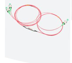
The Polarization Maintaining Tap Coupler is a polarization maintaining coupler which splits the light from the input PM fiber into two output PM fibers. The state of polarization can be aligned either with the slow axis or the fast axis of the PM fibers. The rugged stainless-steel package is designed for high optical performance and stability. This compact device offers low excess insertion loss, low back reflection, and high extinction ratio. Split ratios from 1% to 50% are available.
