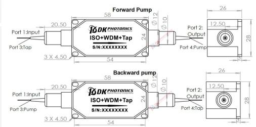
\* For forward pump, Tap is both axis working. For backward pump, Tap is fast axis blocked, slow axis working. Both types pump is both axis working.
