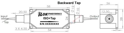
PS: For forward tap, signal wavelength is polarization dependent. For backward tap, signal wavelength is Polarization independent.
